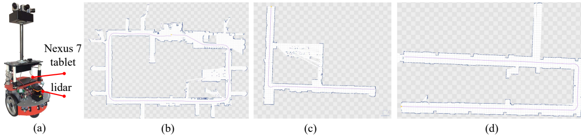
Figure 6.5: (a) Our data collection robot and sensor configuration. 2D lidar maps are used as ground truth: (b) HRBB, (c) SCTS, and (d) WEB. Reprinted with permission from [59].
