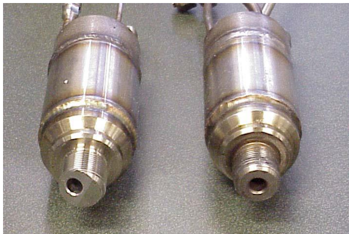
Figure 14: Nozzle with 20 degree angle from PCC centerline (line) and nozzle along PCC centerline (right). Reprinted from [4].
