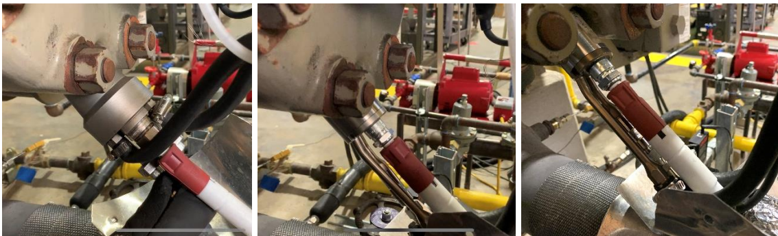
Figure 29: P1 (left), P2 (middle), and P3 (right) installed on the Ajax E-565 engine.
