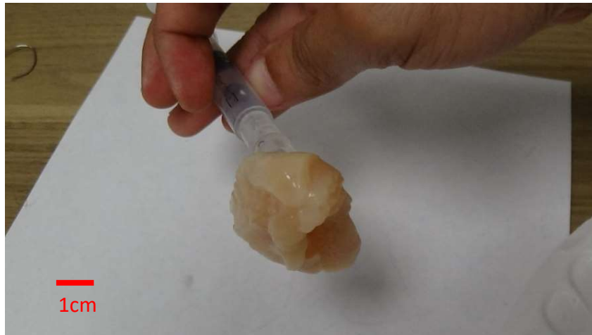
Figure.43. A piece of chicken breast is manipulated to mimic internal organ manipulation. As it can be seen, the hand-like device is holding a piece of chicken breast.
