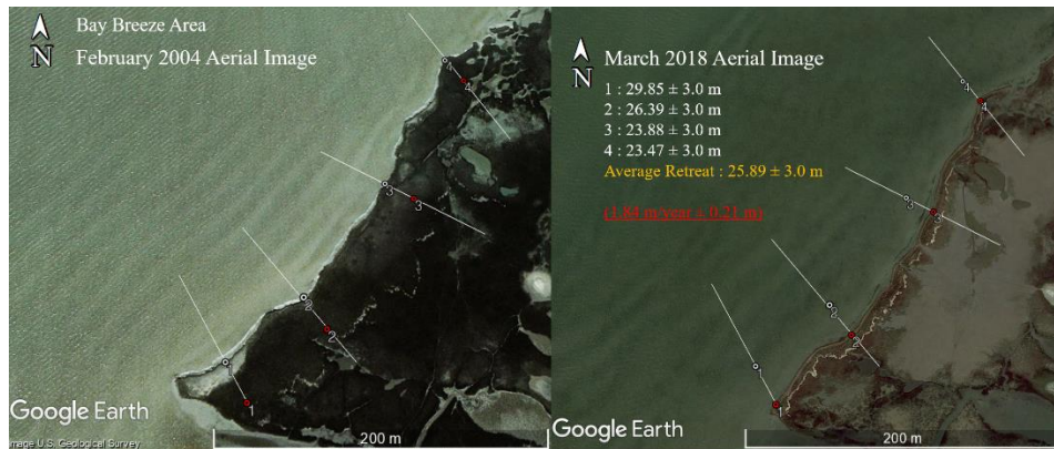
Figure 4-2 Lateral erosion of the Bay Breeze area from Feb 2004 to Mar 2018
