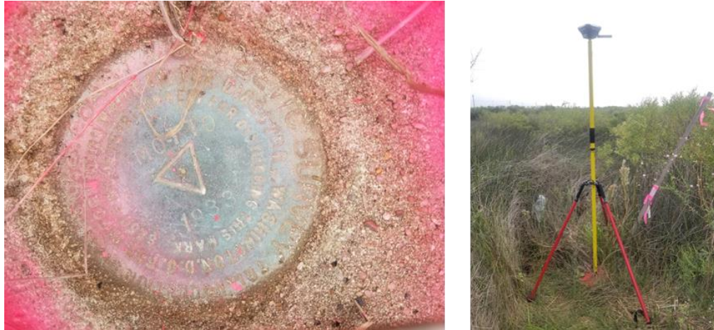
Figure 4-6 MOTTO Station (GCP) by the National Geodetic Survey and installed base GPS on the MOTTO station
