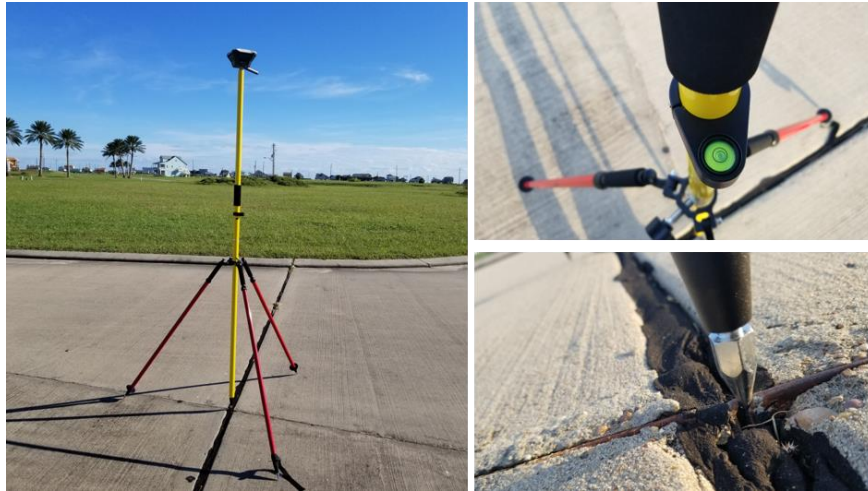
Figure 4-7 The process of the base GPS location on the fixed location in every drone survey
