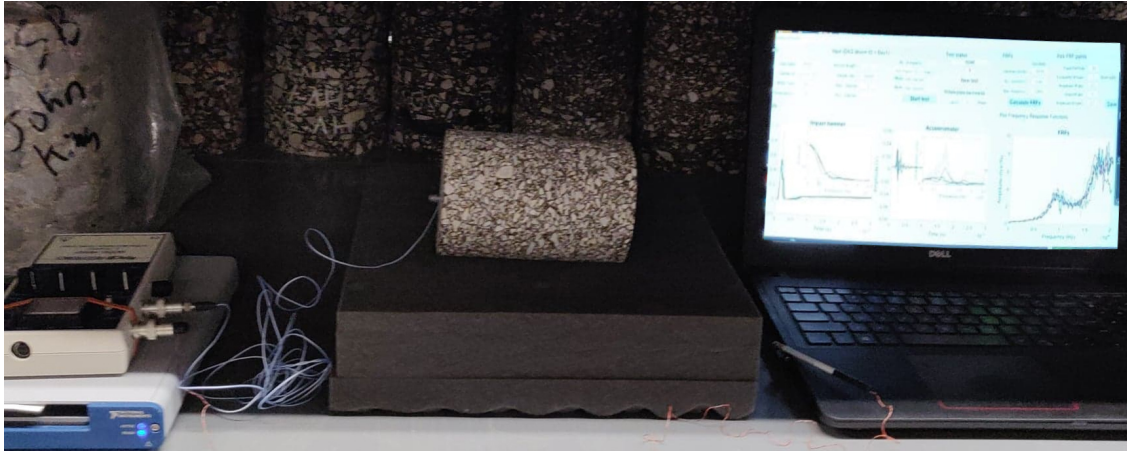
Figure 2-2 Equipment Used to Perform Resonance Testing
