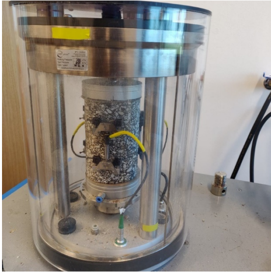
Figure 2-1 Asphalt Mixture Performance Tester Setup
