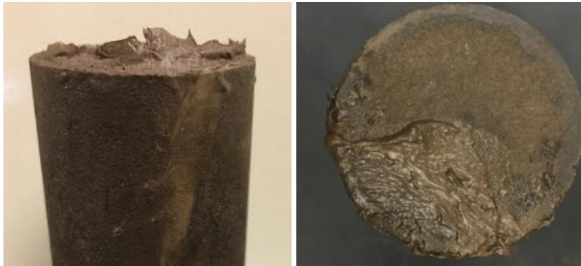
Figure III-9 A Berea sandstone core surface (left) after initial filter cake formation (Experiment 7) and (right) after flowback and final permeability measurements. Reprinted with permission from (Ibrahim et al. 2020).
