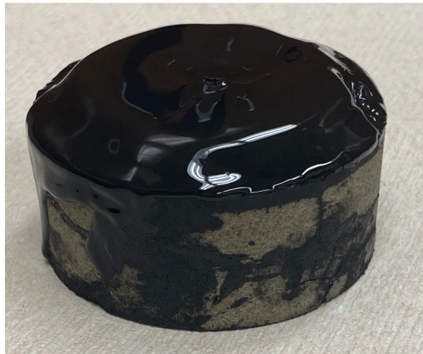
Figure IV-18 The filter cake used in the solubility test with the 10 wt% glycolic and 11.6 wt% citric acid system.
