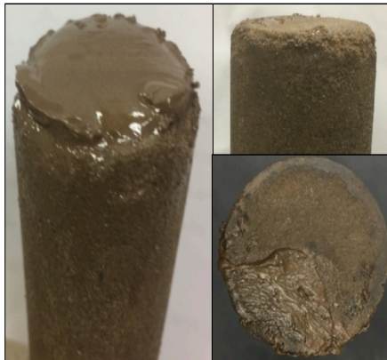
Figure III-5 Dynamic filtration results of Experiment 4 at a 400-psi overbalance. Images show the core surface after initial filter cake formation (left) and after flowback and final permeability measurements (right). Reprinted with permission from (Ibrahim et al. 2020).
