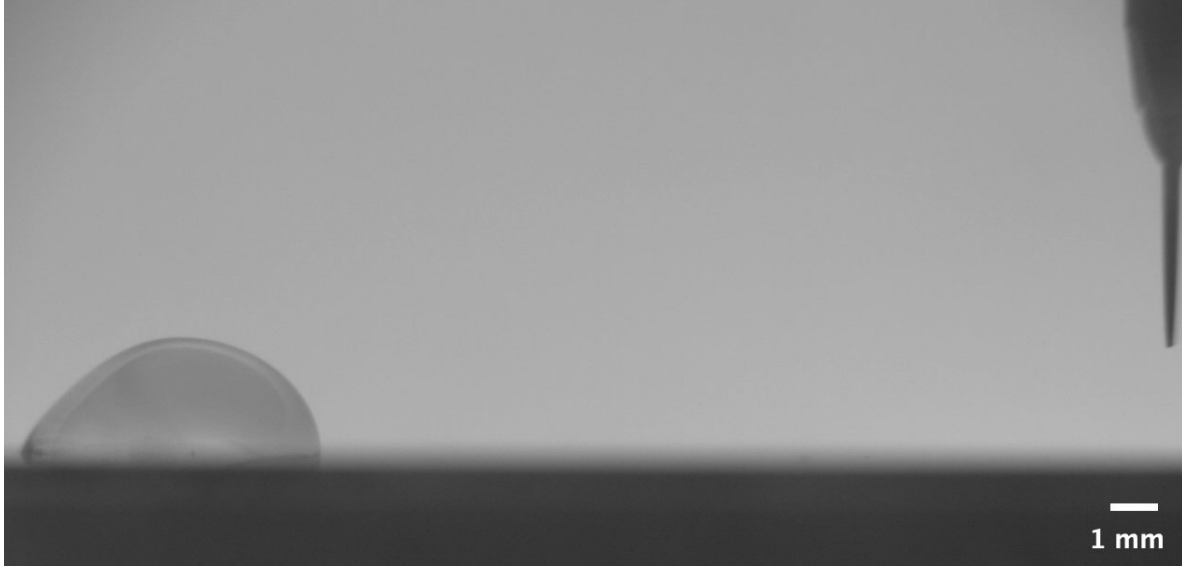
Figure 4.5: Shape of 50 \mu\text{L} water drop at 7.9 m/s and hotwire location relative to drop advancing side
