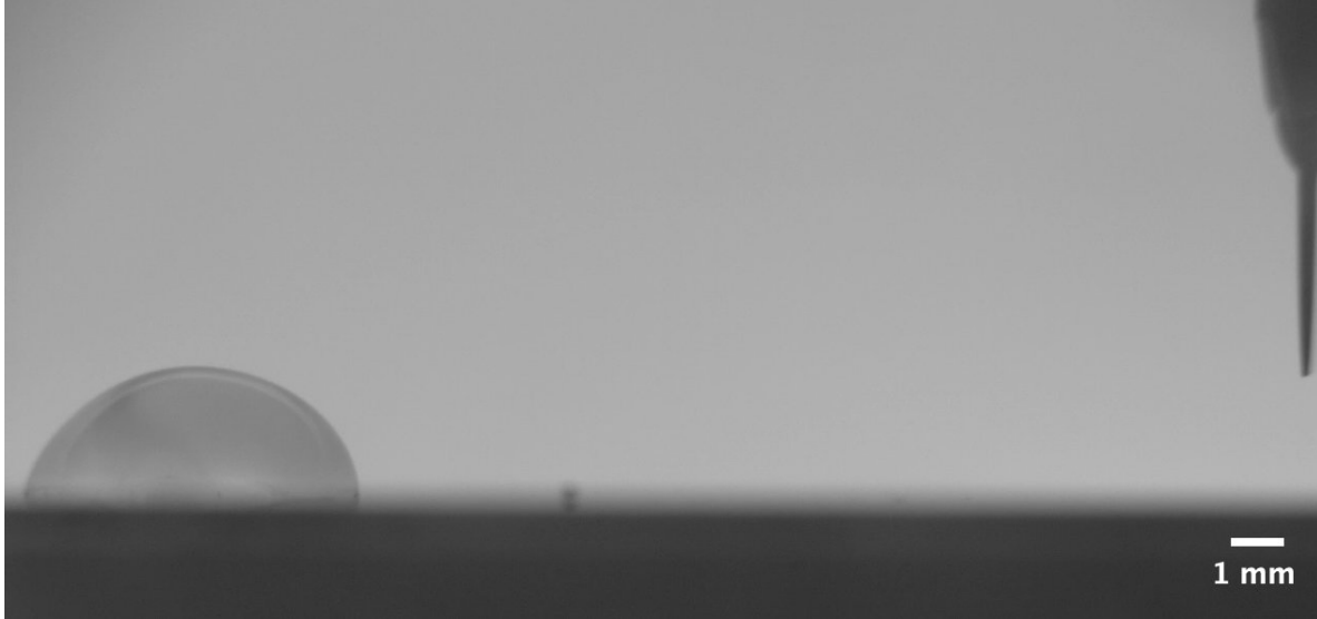
Figure 4.3: Shape of 50 \mu\text{L} water drop at 5.9 \text{ m/s} and hotwire location relative to drop advancing side
