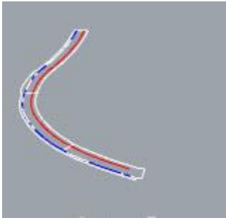
Figure 34. frame curvature used to develop planking profile (Drawing: M. Lewis)
