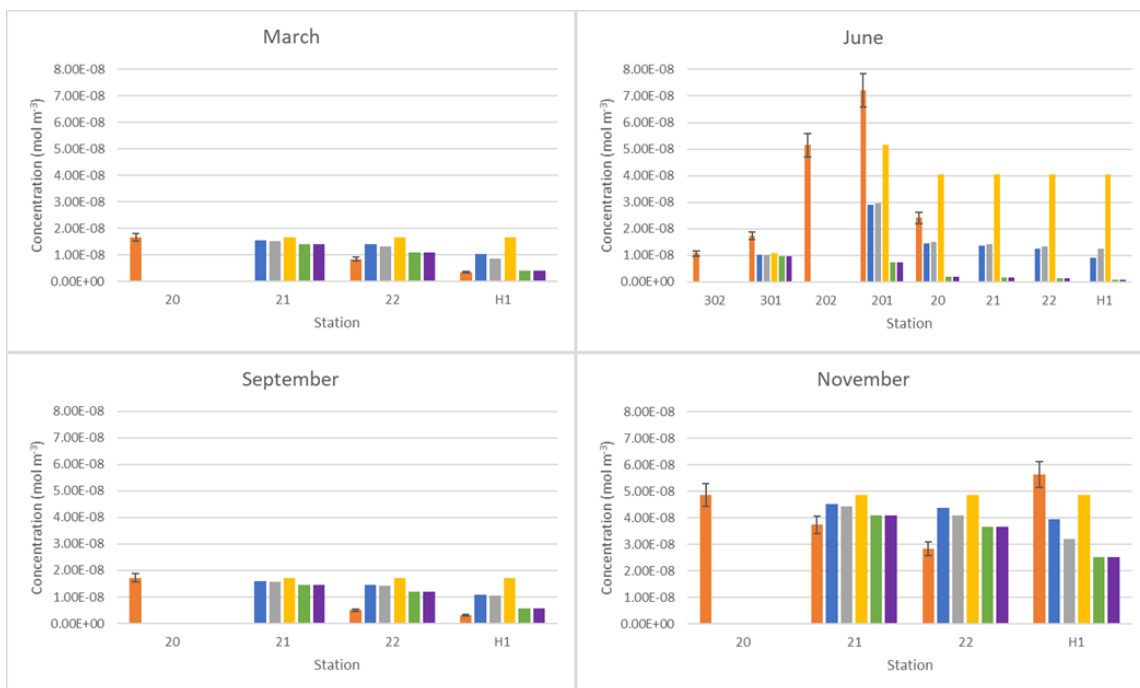
Figure 18: The projected concentrations of PCE using known loss parameters for March, June, September, and November 2019. Orange is the observed concentration measured on station, blue is the concentration if air-sea flux was the only loss parameter, gray is the concentration if mixing to depth was the only loss parameter, yellow is the concentration if only hydrolysis was the loss parameter, green is the concentration from loss by air-sea flux and mixing to depth, and purple is the concentration from loss with flux, mixing, and the loss rate of PCE at the surface from Ambrose (1987).
