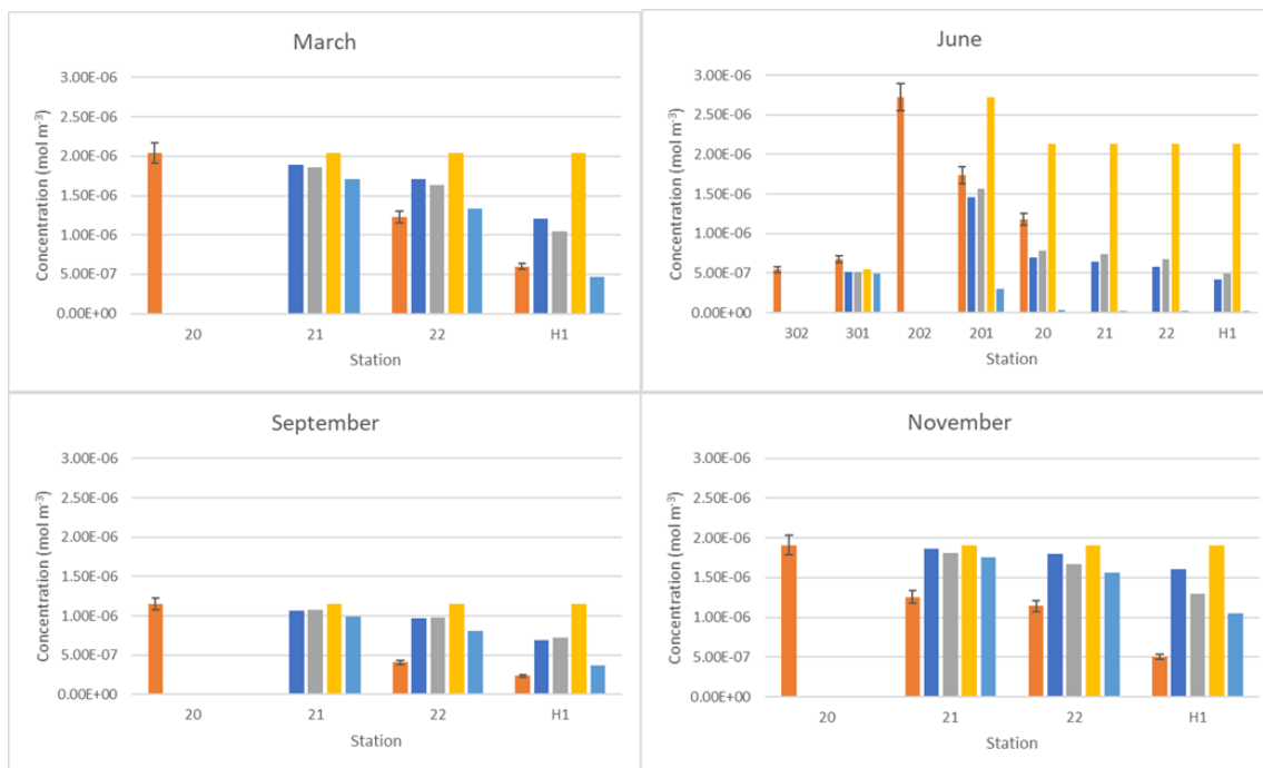
Figure 16: The projected concentrations of \text{CHCl}_3 using known loss parameters for March, June, September, and November 2019. Orange is the observed concentration measured on station, blue is the concentration if air-sea flux was the only loss parameter, gray is the concentration if mixing to depth was the only loss parameter, yellow is the concentration if only hydrolysis was the loss parameter, and light blue is the concentration from loss by air-sea flux and mixing to depth.
