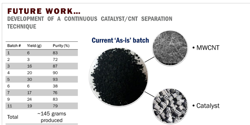
Figure 6.2 Targeting a continuous MWCNT/catalyst separation and recycle system for catalyst reuse while improving MWCNT purity
