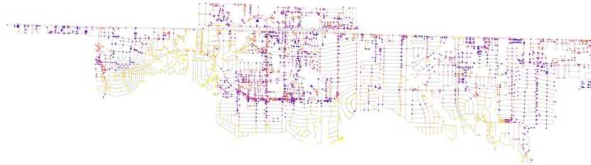
Figure 67 Color map for the cumulative inundation values of nodes (yellow represents high values; purple represents low values)
