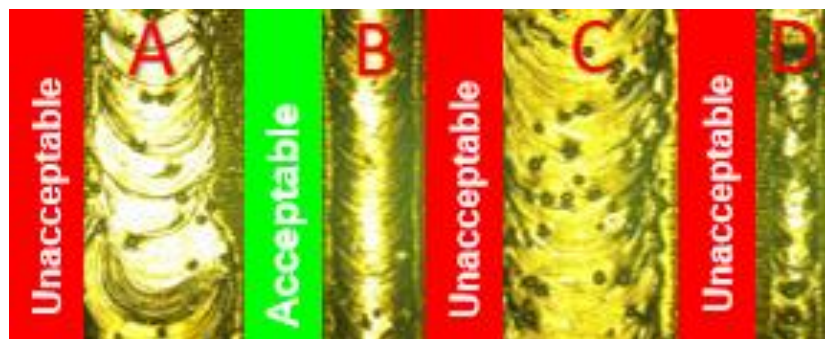
Figure 17. (a) Selected single tracks of Cr printed using the DED system with the power and speed combinations shown. The four tracks in (b) are from the red boxes in (a) displaying the classification of acceptable and unacceptable tracks. A is an example for non-uniform track width; B: Acceptable, good track; C: Uneven solidification front and spatter particles; D: Lack of sufficient fusion to the substrate.
