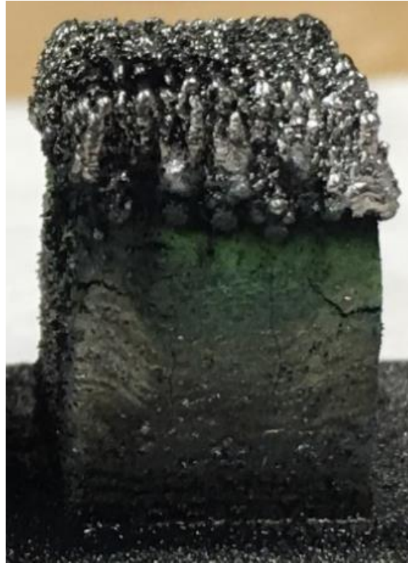
Figure 24. Full gradient print of the designed Path from Fe-9Cr to 100 %W.
