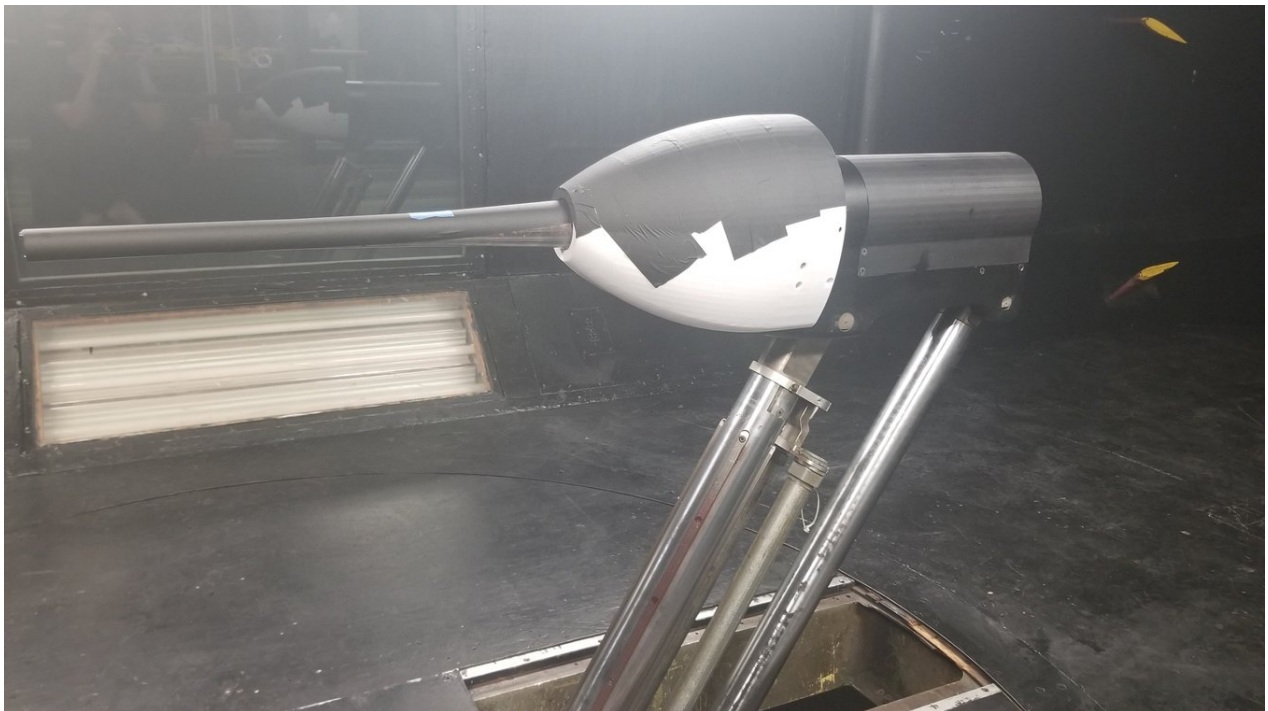
Figure 4.1: 2014 bullet fairing installed on new HARS bullet for PIV data capture
