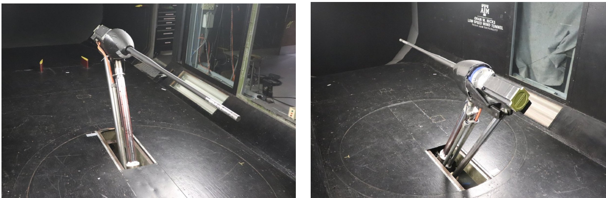
Figure 1.2: 2014 HARS system installed in LSWT test section
