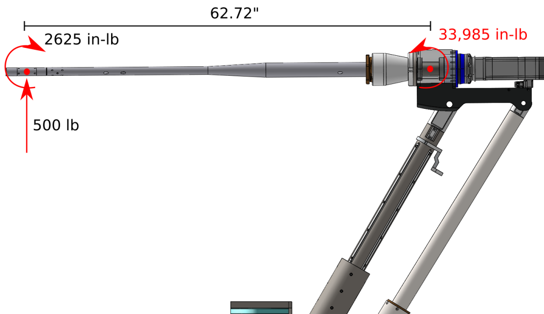
Figure 3.1: Free-Body Diagram of HARS resultant moment from maximum-loaded internal balance on 55.5-inch sting.
