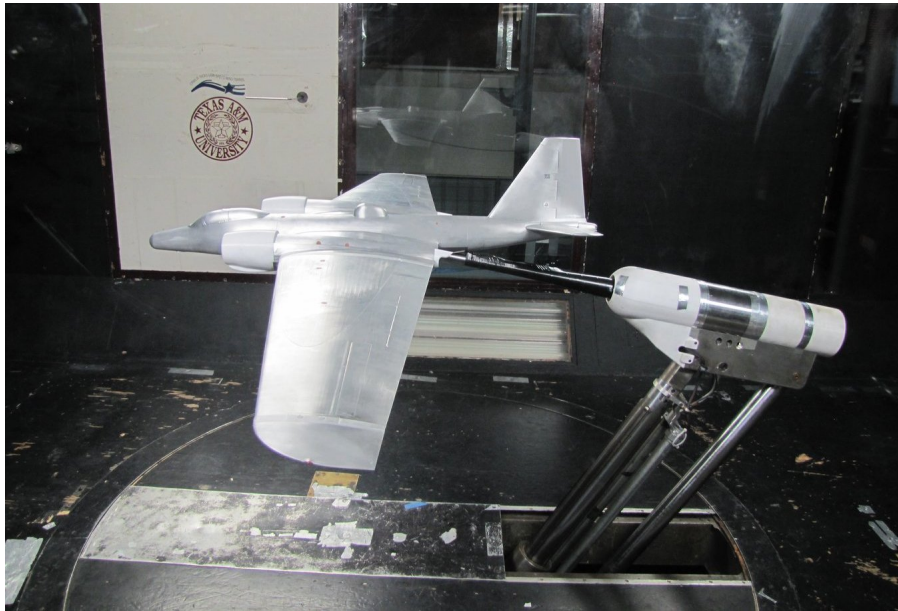
Figure 2.2: 2009 HARS system installed in LSWT test section with WB-57 model
