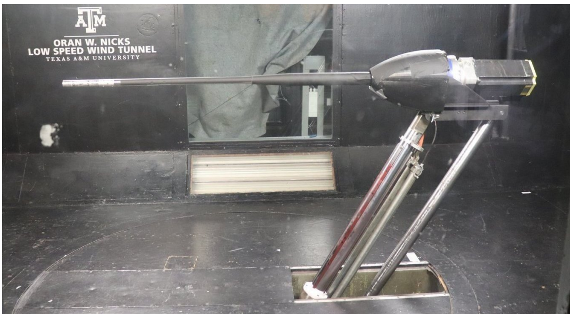
Figure 1.1: HARS system installed in LSWT test section with 55.5-inch sting
