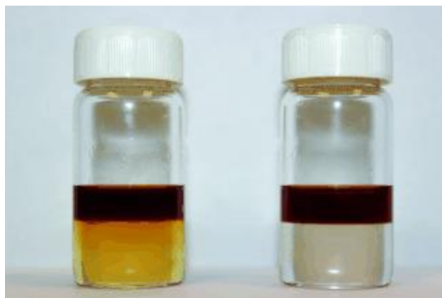
Figure I-34 Visualization of the anti-leaching effect of PIB 2300 . In a heptane/ethanol/DMF solvent system, PIB bound ruthenium bipyridine has partial leaching into polar phase (left). In the same solvent system, with addition of PIB 2300 cosolvent, the leaching of the PIB bound ruthenium is greatly decreased (right). Reprinted with permission from (57).
