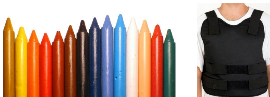
Figure I-3 Low MW PE used for soft coloring materials and UHMWPE used as body armor
