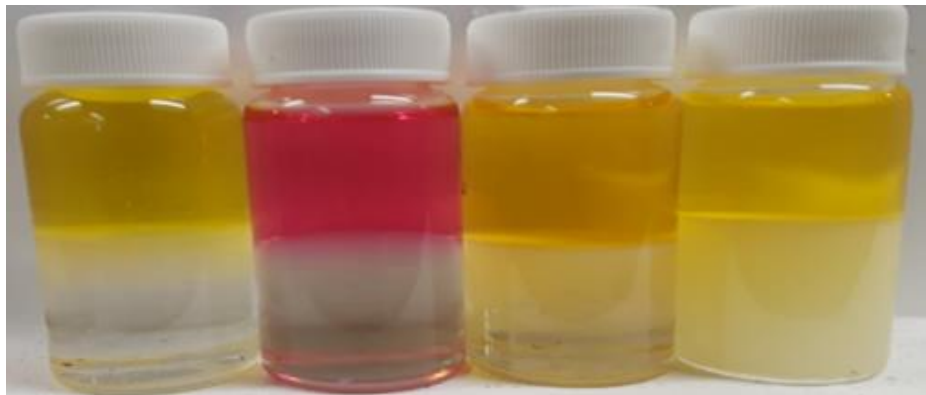
Figure III-15 (far left) p -Methyl red 4 dissolved into methanol above a PAO 432 phase while, (second from left) p -methyl red 4 dissolved into methanol with methanesulfonic acid above a PAO 432 , (second from right) p -methyl red 4 dissolved into methanol above a PAO 432 phase containing 2 and (right) p -methyl red 4 dissolved into methanol above a PAO 432 phase containing 3 .
