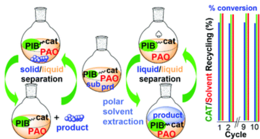
Figure I-38 Product isolation methods from PAOs. Reprinted with permission from (60).
