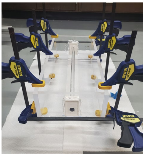
Figure 3.20 Experimental Set-up to determine the natural frequency, f_N , of the system
