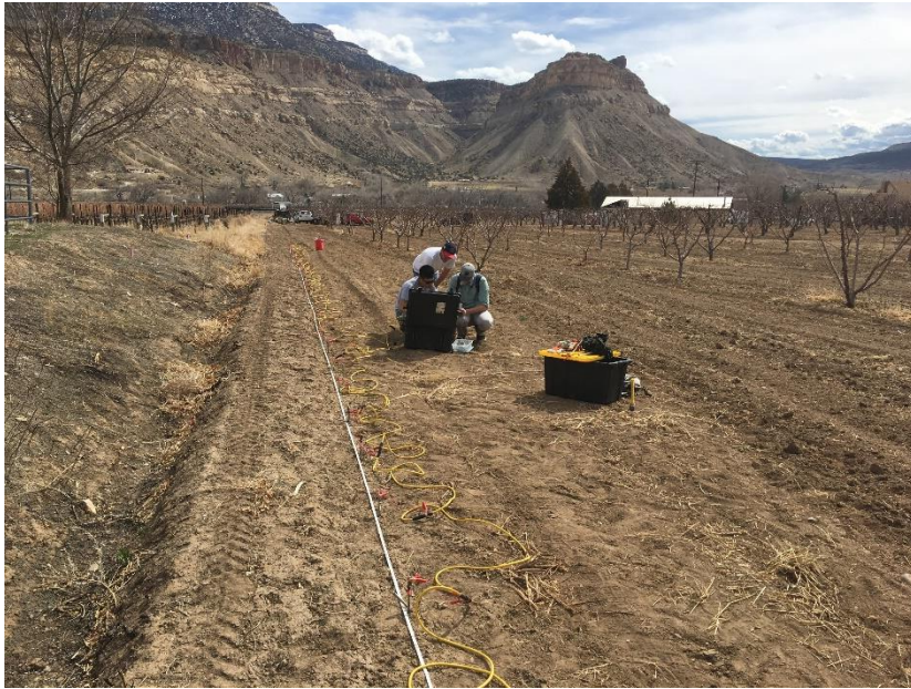
Figure 3.3 A Field Setup of a Dipole-Dipole Survey of ERT.
