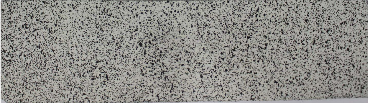
Figure 62 Random contrasting speckle pattern applied to a specimen for DIC purpose.
