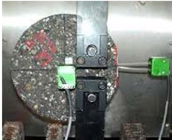
Figure 3. Disk-shaped compact test set-up (reprinted from Wagoner, Buttlar et al. (2005)).
