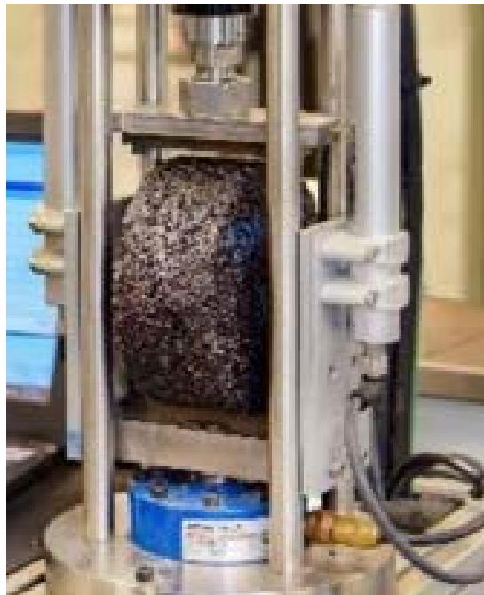
Figure 5. IDEAL-CT test set-up (reprinted from Zhou (2019)).
