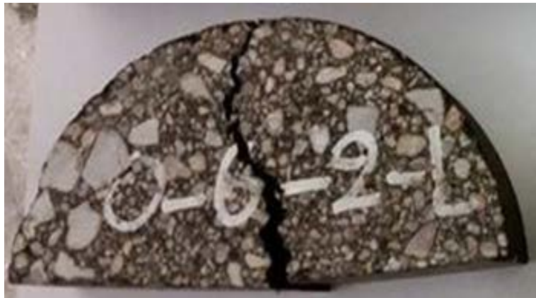
Figure 28. Off-center crack initiation for notch-less SCB specimens.
