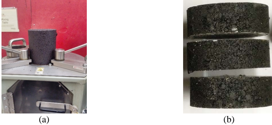
Figure 44. SCB sample preparation: (a) compaction by SGC and (b) slicing.
