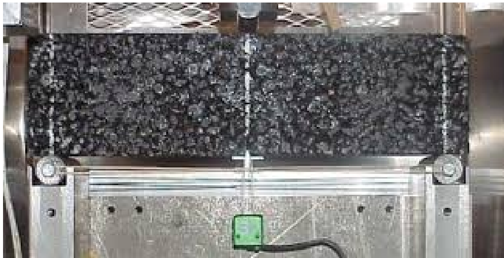
Figure 6. SENB test set-up (reprinted from Wagoner, Buttlar et al. (2005)).
