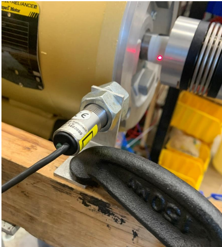
Figure 3.7: Tachometer used to measure turbine speed during operation shown in its operational position during testing.
