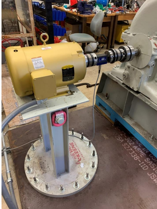
Figure 3.2: Picture of the motor stand secured to base plate by threaded steel rods and nuts.
