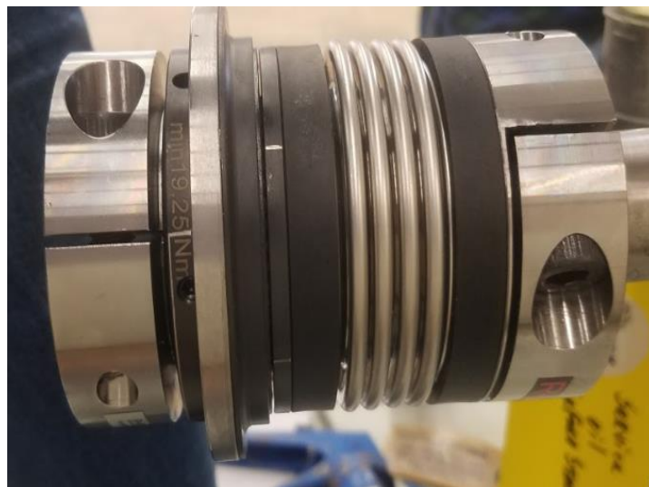
Figure 3.4: SK2 safety coupling used to attach torque meter to Terry Turbine.
