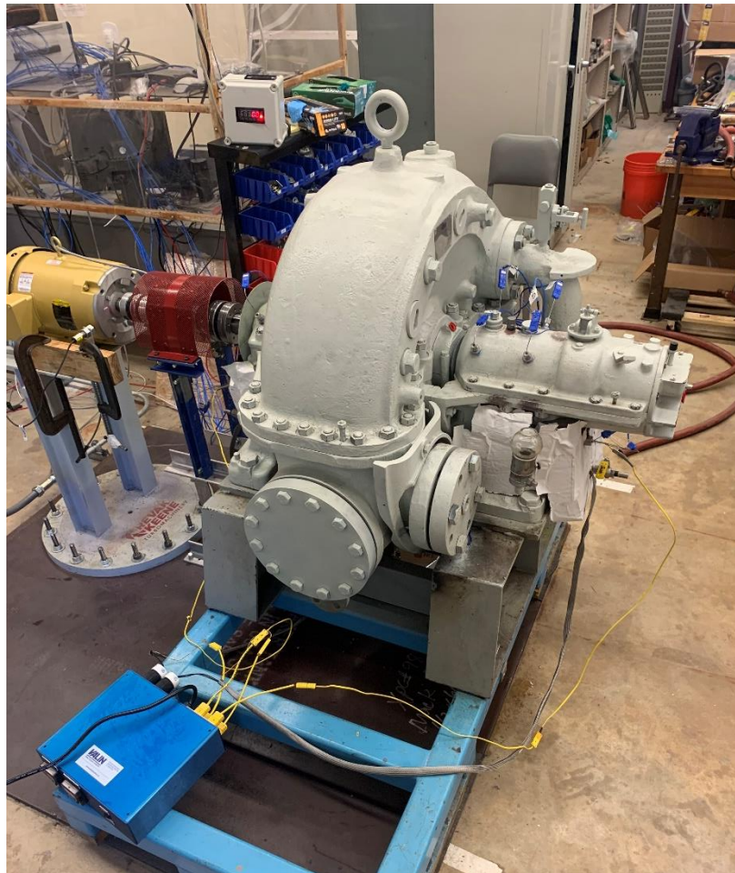
Figure 3.20: Whole turbine test facility with heater control console and shaft blast guard.
