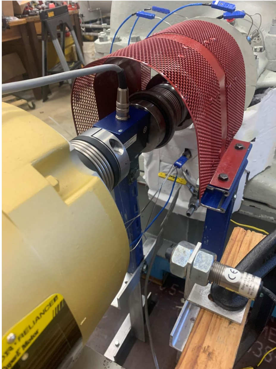
Figure 3.22: View down the facility shaft with torque meter in vertical orientation as tested.
