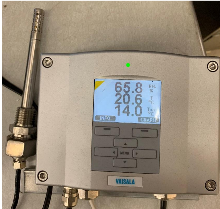
Figure 3.9: Hygrometer with power supplied showing atmospheric conditions of the Laboratory for Nuclear Heat Transfer Systems.
