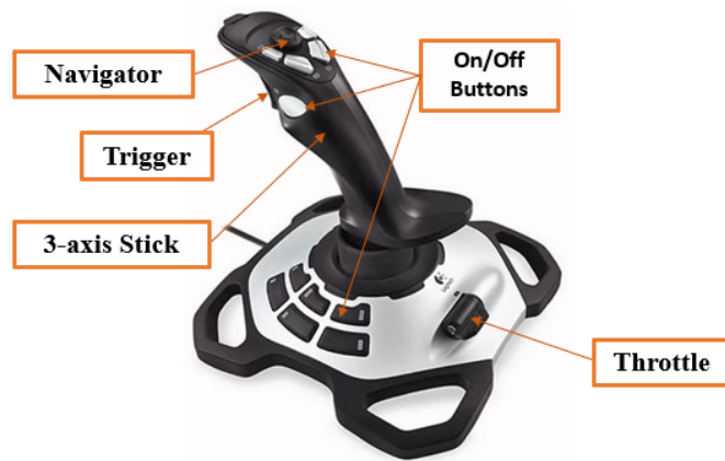
Figure 2.3: General Purpose Joysticks and Common Features
