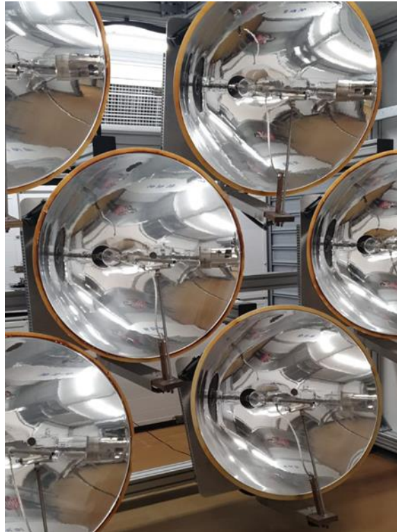
Figure 12: Xenon Arc Lamps Concentrating Light
