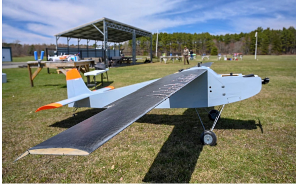
Figure 1.6: Physical custom built hardware test-bed whose digital twin is used for this research
