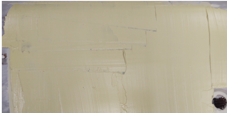
Figure 7.4: Blade with putty before sanding
