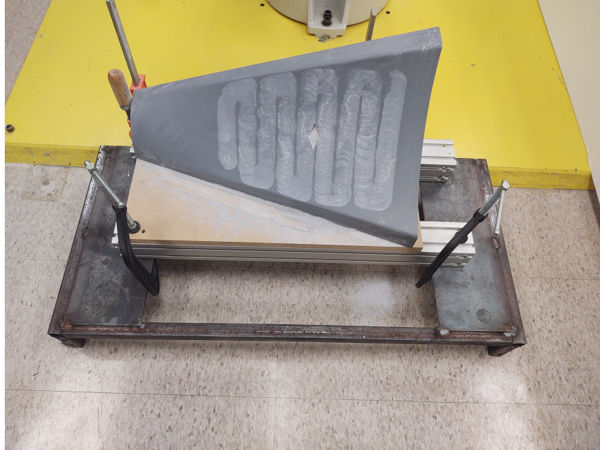
Figure 7.9: Concave surface with uncovered strips between passes
