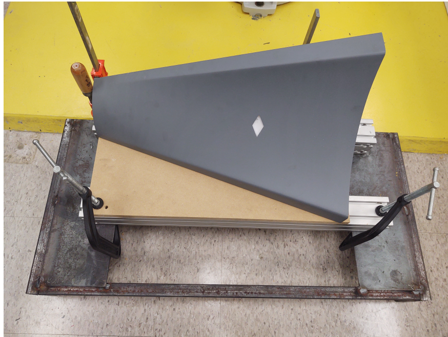
Figure 7.6: Concave surface before sanding
