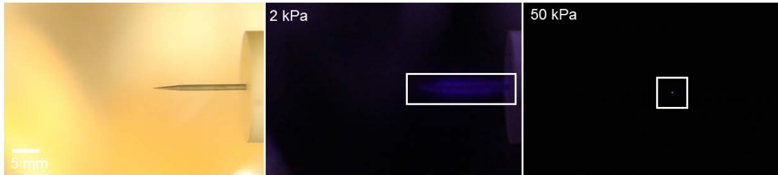
Figure 3.10 Images for pulsed discharges (white box) in air at sub-atmospheric pressure. Here, SG1 = 6 mm and SG2 = 2 mm. Exposure time of image is 1 s. Images are accumulation of \approx 3 pulses.
