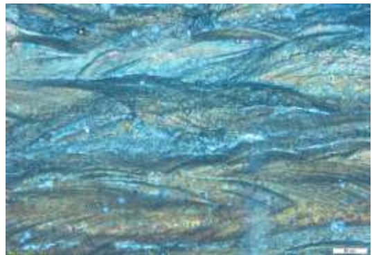
Figure 5-1-7: Microscope Image 20X (1400 J/mm^3 )
