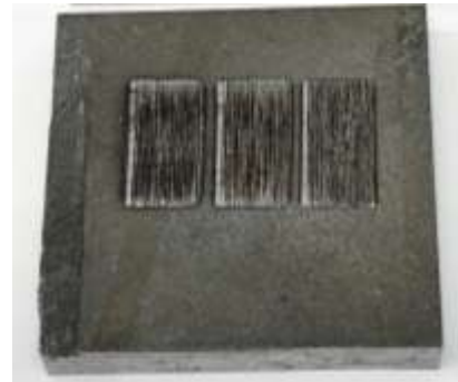
Figure 6-1-2: H13 Lapped Substrate (950, 1100, 1250 J/mm 3 )
