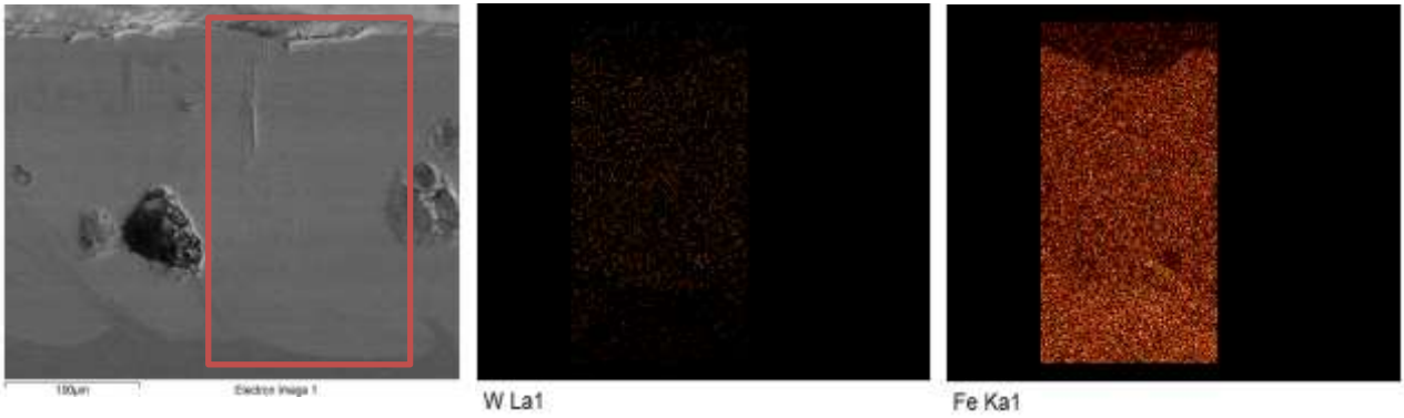
Figure 5-2-14: W and Fe Distribution within the Cross-Section ( 1400 J/mm^3 )
