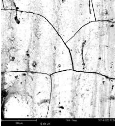
Figure 6-3-20: Lapped H13 SEM Image ( 500 \text{ J/mm}^3 )
