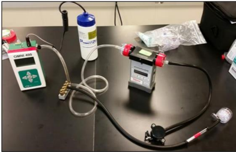
Figure 3.1 Backpack and Personal Air Monitoring Devices: Pump and PDR with Battery pack
