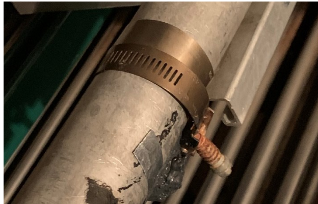
Figure 15: Hose clamp for connection of K type thermocouples
