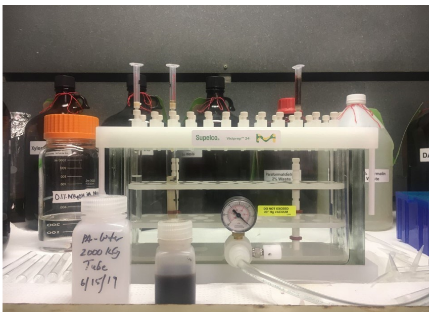
Figure 22: Solid phase extraction (SPE) manifold for concentrate and purify sample
