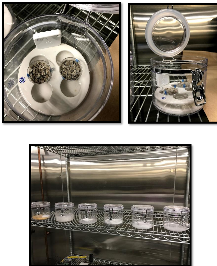
Figure A- 1 Crushed samples stored in a desiccator at varying RH environments.
