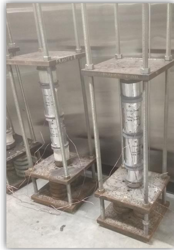
Figure 4-2 Uniaxial concrete creep test setup.
