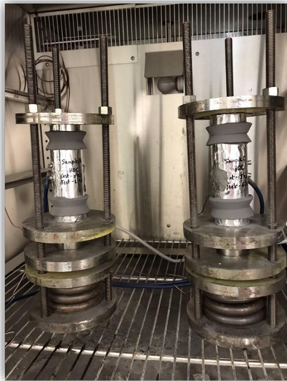
Figure 2-8 Uniaxial creep test setup using the miniaturized creep frame inside an environmental chamber maintaining constant temperature and humidity.
