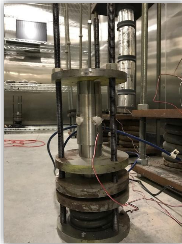
Figure 3-2 Confined creep test setup using the miniaturized creep frame placed inside an environmental chamber maintaining constant temperature and humidity.
