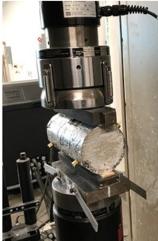
Figure 4-19 Experimental set up of splitting tensile test.
