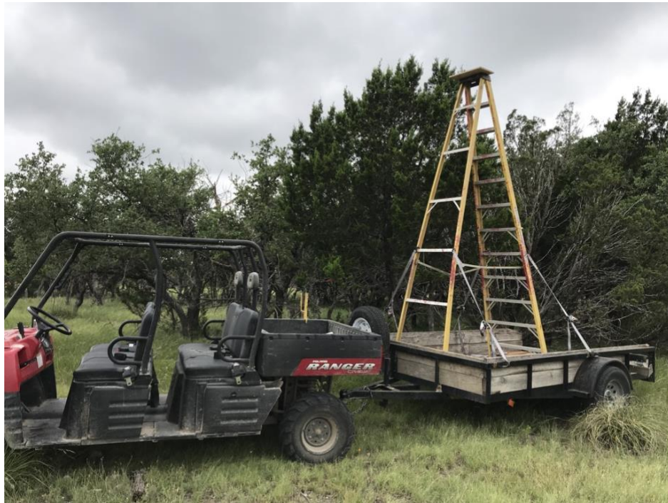
Figure 2.2 Mobile tree sampling platform for leaf-level physiology measurements.
