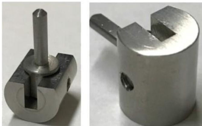
Figure III-1. Self-aligned stainless-steel barrel tip used for mar test. Reprinted from Chrisman et al. [29].
