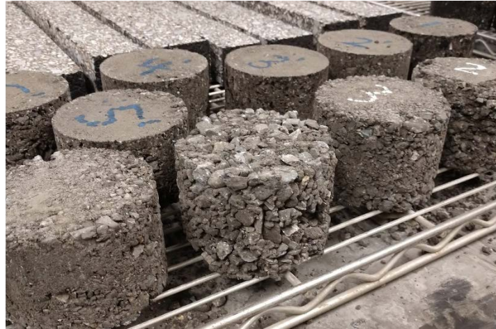
Figure 8 - Delaware specimens conditioned at 70°C and compacted with the SGC (rear) and Marshall apparatus (front)
