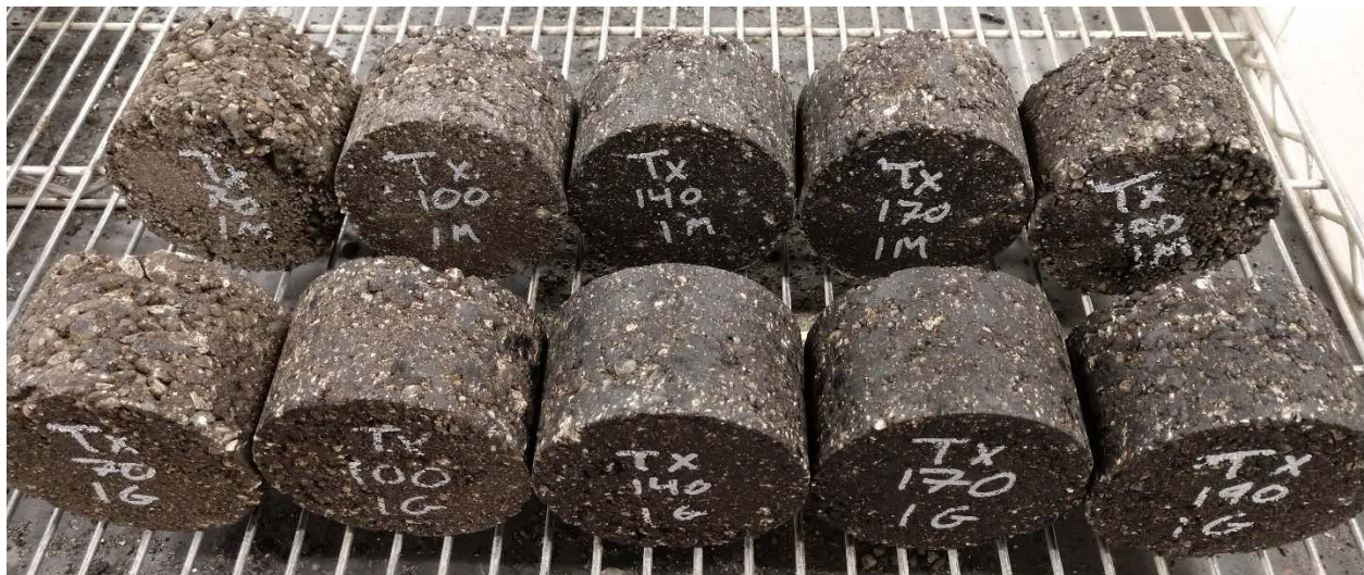
Figure 22 - Texas RAP conditioned at all temperatures and separated by Marshall compaction (rear) and SGC compaction (front)
