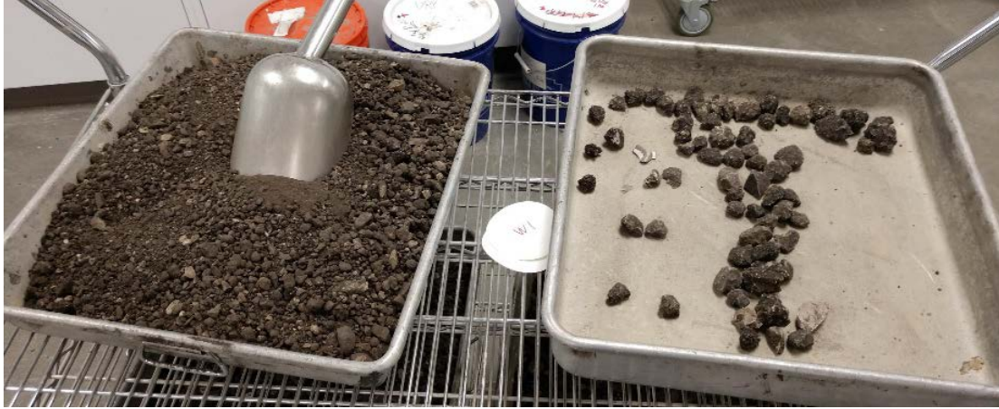
Figure 6 - Uncompacted Florida RAP, passing 3/4" on the left, and retained on 3/4" on the right
