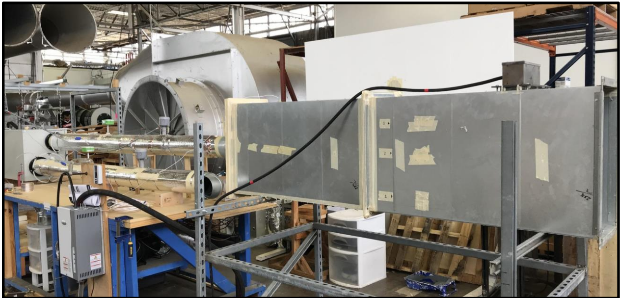
Figure 3. Section of test setup connected to immersion heater
