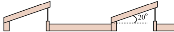
(c) Vertical roof monitors facing north and clear glazing Vertical roof monitors facing south and diffuse glazing
