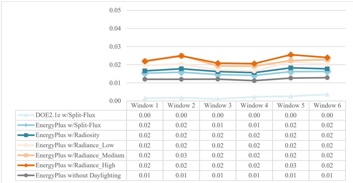
Figure 4.49: Annual Heating Load Use with Floor Visual Reflectance 0.5 (West Facing Window, Phoenix, AZ)
