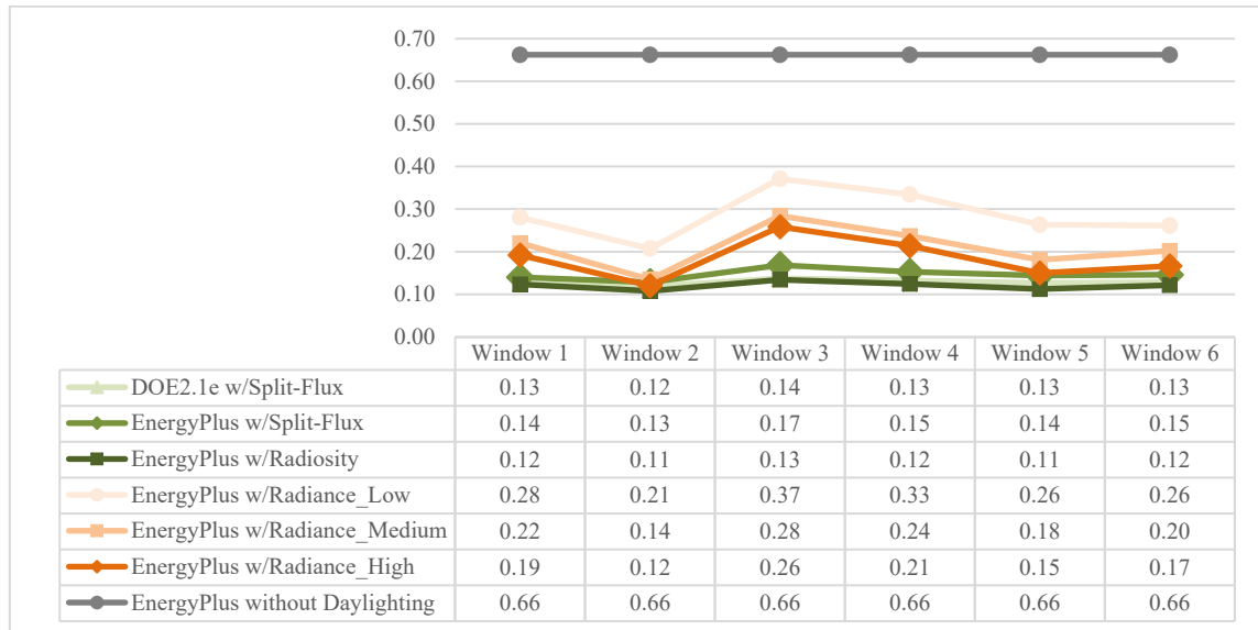
Figure 4.26: Annual Lighting Energy Use with Floor Visual Reflectance 0.2 (East Facing Window, Phoenix, AZ)
