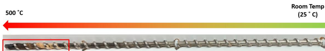
Figure 8. Screw feeder as received with severe biomass accumulation towards the tip
