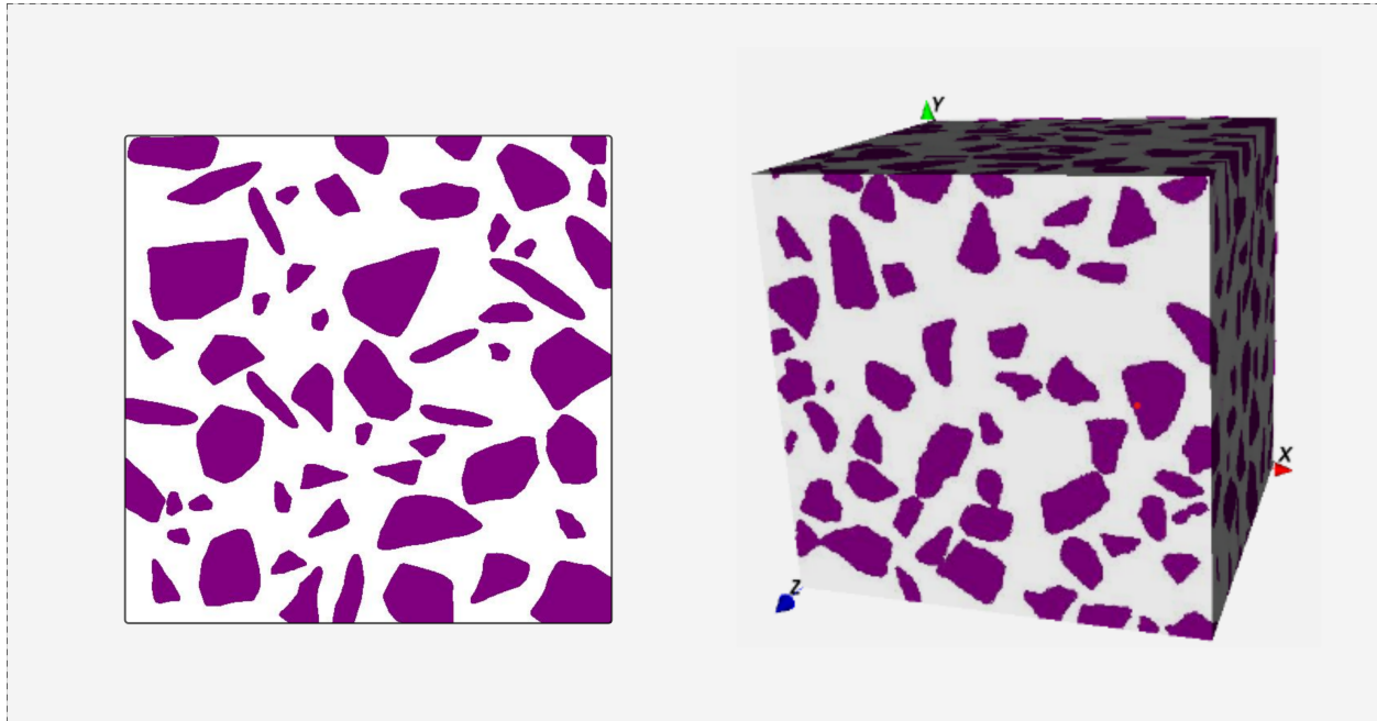
Figure 3.5: A 2D microstructure (left) and a 3D microstructure (right) with cored boundary conditions composed of 38% coarse aggregates by area and volume, respectively.
