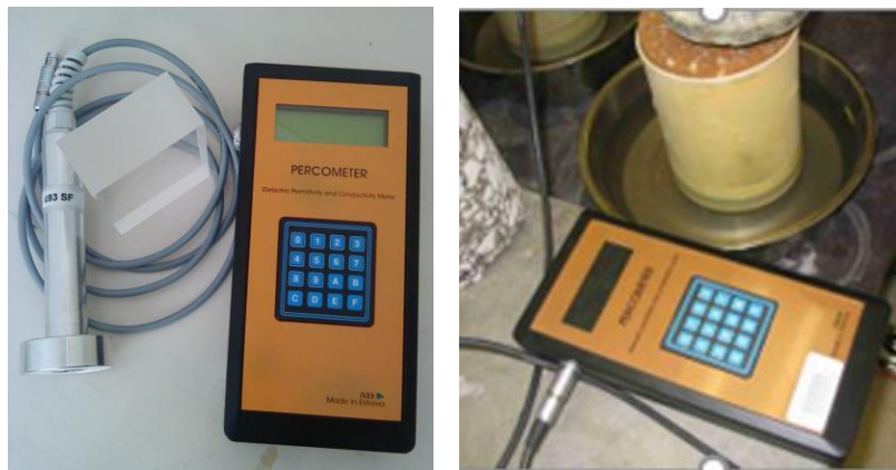
Figure 6. Percometer to Measure the Dielectric Constant of Soil Surface
