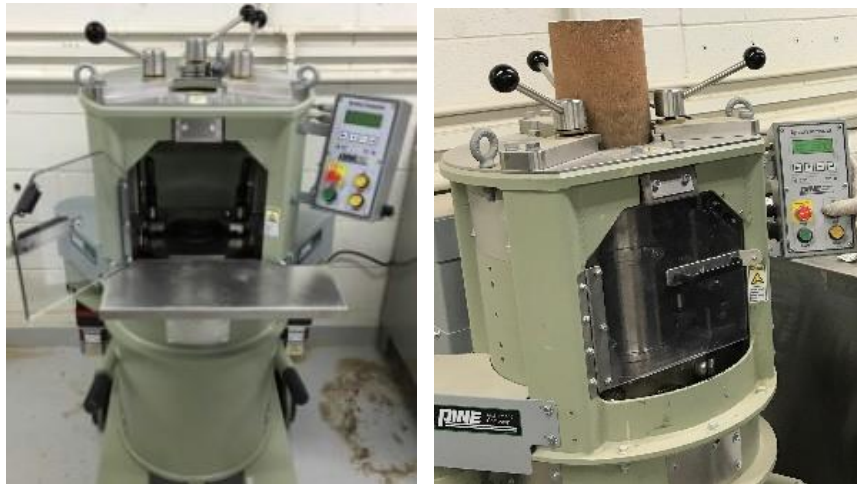
Figure 2. Superpave Gyratory Compactor Used in this Research for Compaction of Granular Materials
