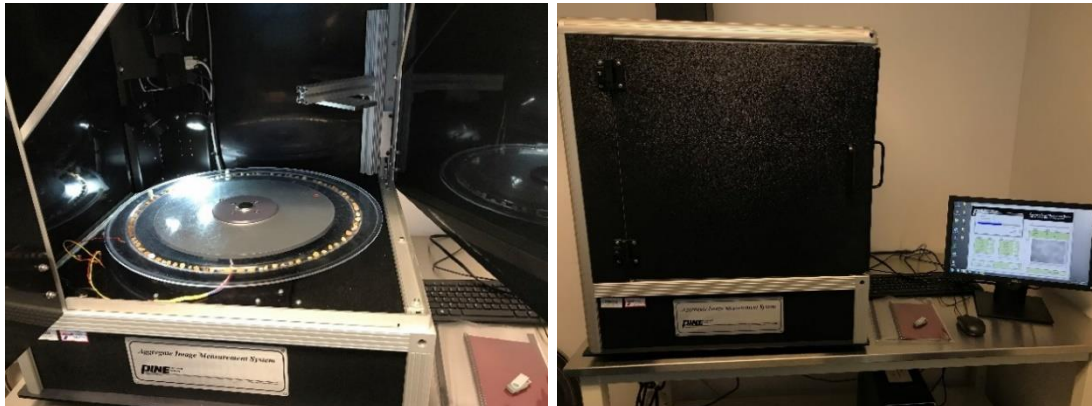
Figure 7. Aggregate Imaging System (AIMS) Device Used in This Study
