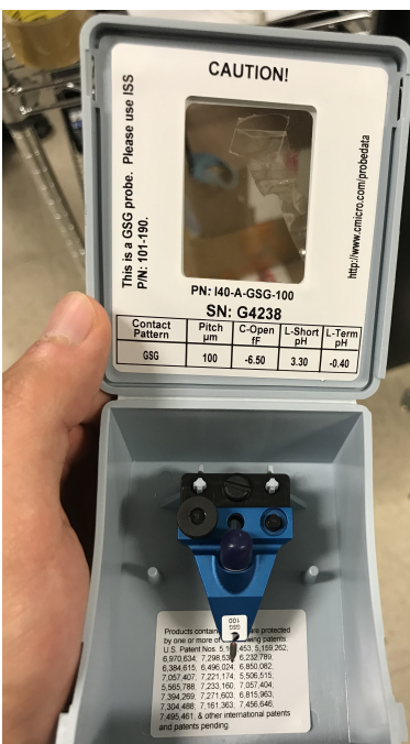
Figure 3.28: The used GSG probe in the protecting package.
