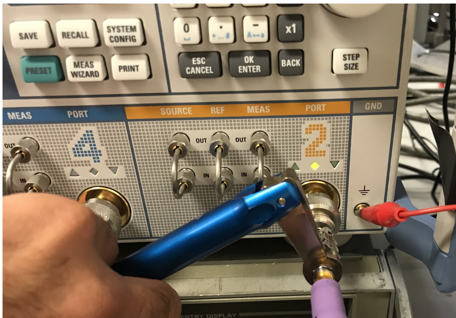
Figure 3.34: The bias tee and connection to the VNA input.
