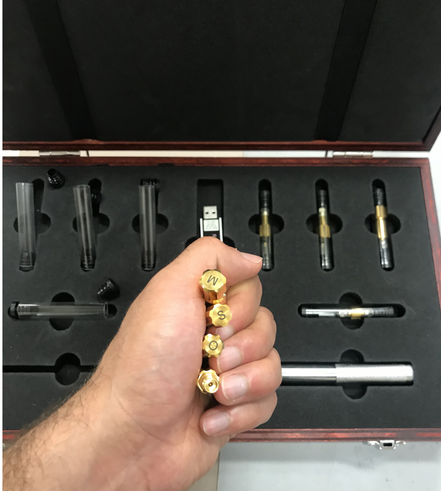
Figure 3.36: The calibration terminations (loads) of the VNA.
