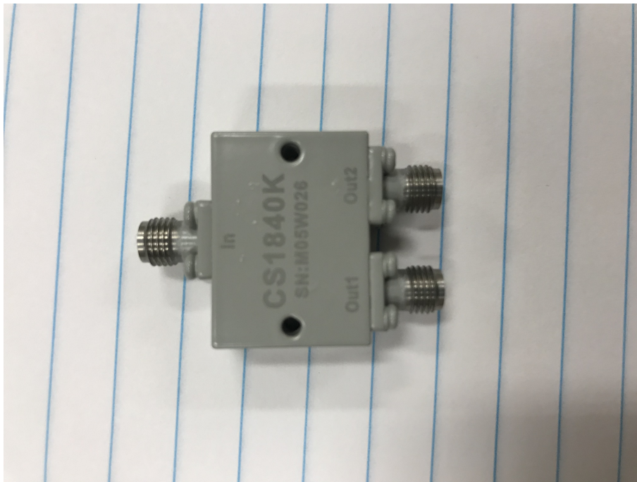
Figure 3.42: The commercial power combiner and divider (CS1840K).
