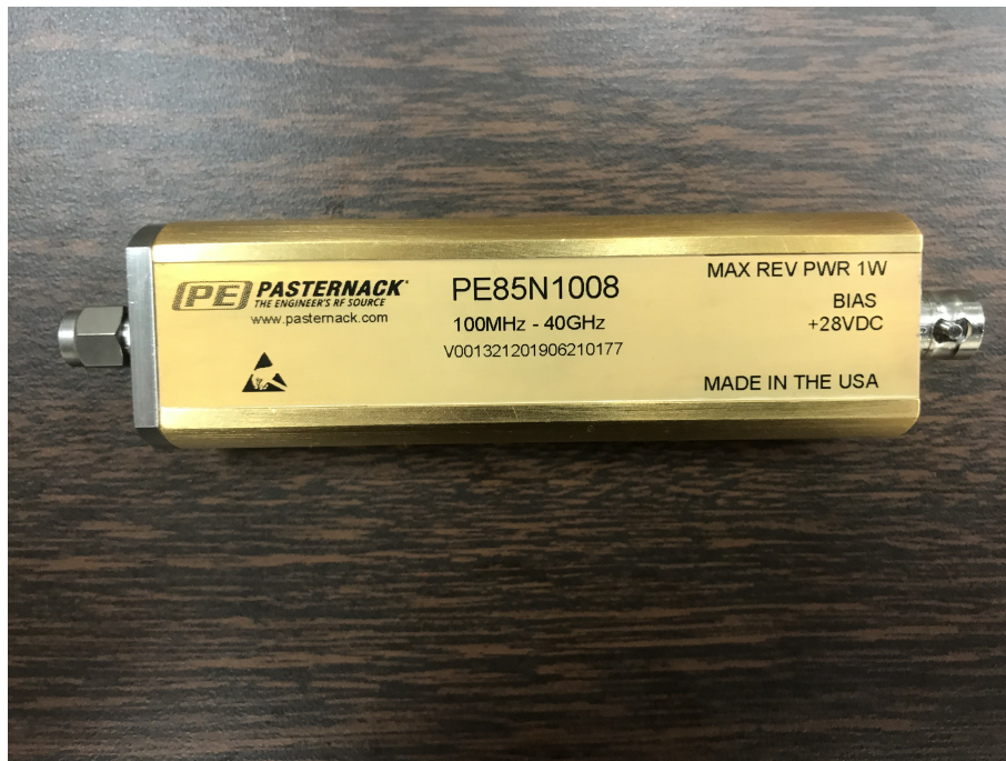
Figure 3.38: The commercial 1-40 GHz noise source.
