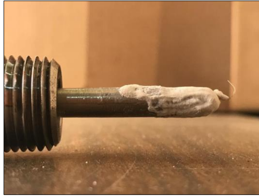
Figure 19: High speed thermocouple probe.
