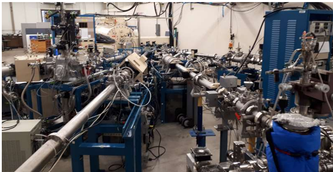
Figure 2.12 Post acceleration switching magnet with extended beamlines.
