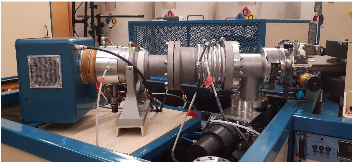
Figure 2.6 RF source without safety cage on a 3MV Pelletron accelerator system.
