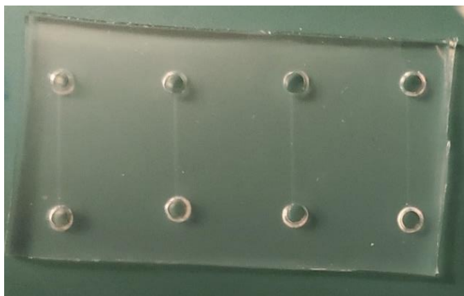
Figure S1. Photograph of a 14% PEO-PDMS microfluidic chip bonded to a glass slide.
