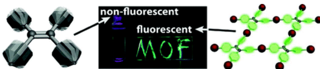
Figure I-4. Turn-On Fluorescence of TCPE by Coordination in a Rigid MOF Matrix (MCIE). Reproduced with permission from J. Am. Chem. Soc. 2011, 133, 50, 20126-20129. 64 Copyright 2011 American Chemical Society.
