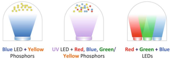
Figure 3. Illustration of white light generation using phosphor method (blue/UV LEDs + phosphors) and using RGB method (Red+Green+Blue LEDs). 15 (Reprinted with Creative Commons Attribution 4.0 International Public License from Ref. 15. Copyright 2016 Springer.)
