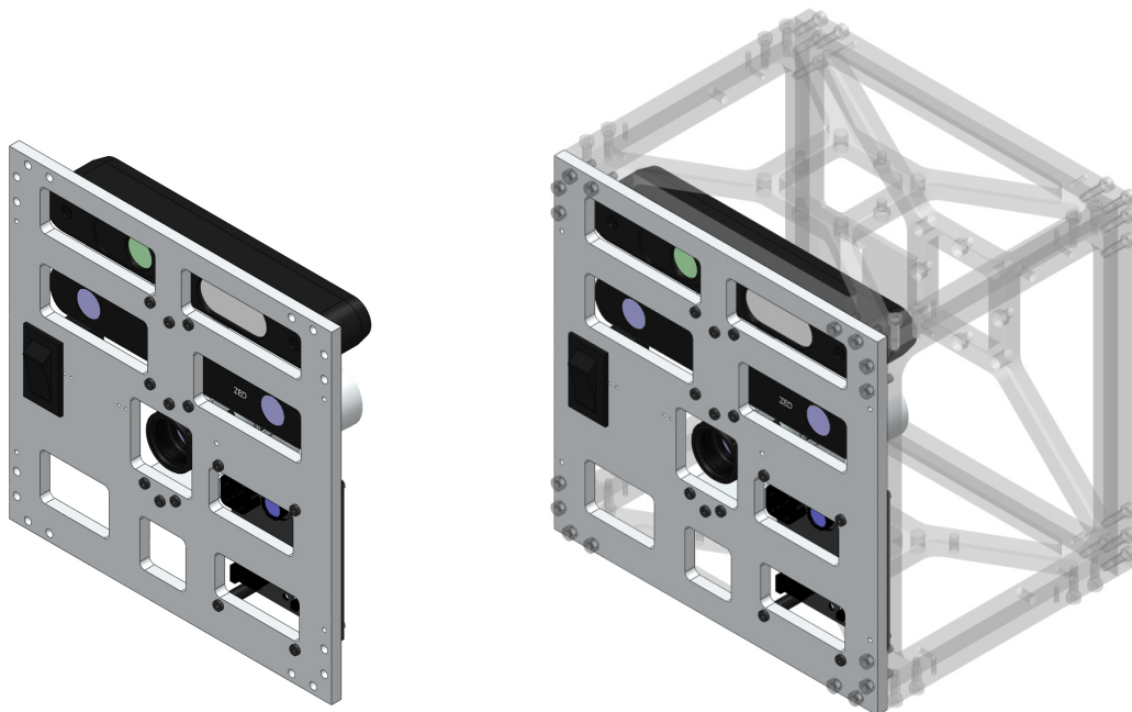
Figure 5.4: Isometric view of the sensor array subassembly (left); the sensor array subassembly mounted to the chassis with the chassis displayed transparent (right).
