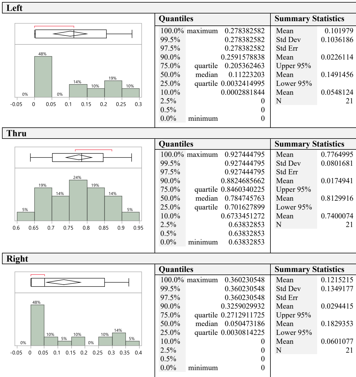
Figure 10 JMP analysis results for partial exclusive and partial shared lane group of a 4 leg intersection with 2-thru (1 shared rt) lanes.
