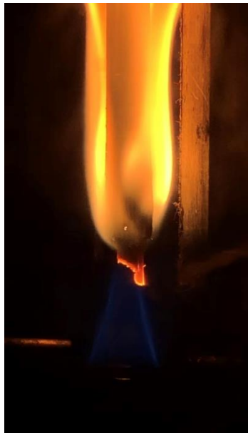
Figure 3.4 Picture of a 21-ply cross-ply Cytec Cycom 5215 T40-800 graphite-epoxy UNC0 specimen during vertical burning test using a Bunsen burner.
