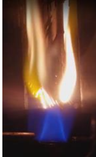
Figure 5.17 Positioning of the IPS specimen during vertical burn tests.
