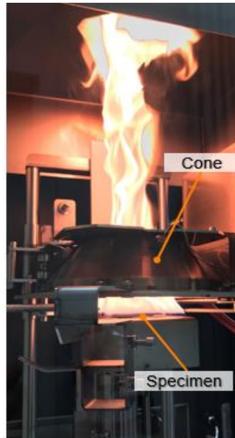
Figure 5.31 Cone calorimetry testing of a 4 x 4 in 2 32-ply Cytec Cycom 5215 T40-800 graphite-epoxy CAI specimen.
