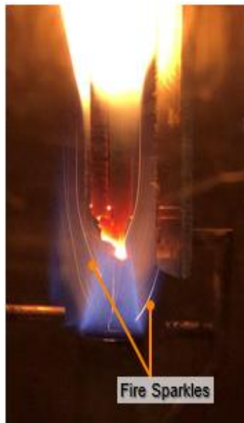
Figure 5.1 Fire sparkles during the 12 s vertical burn test on a 21-ply cross-ply Cytec Cycom 5215 T40-800 graphite-epoxy UNC0 specimen.
