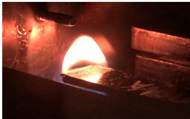
Figure 3.5 Picture of a 21-ply cross-ply Cytec Cycom 5215 T40-800 graphite-epoxy UNC0 specimen during horizontal burning test using a Bunsen burner.
