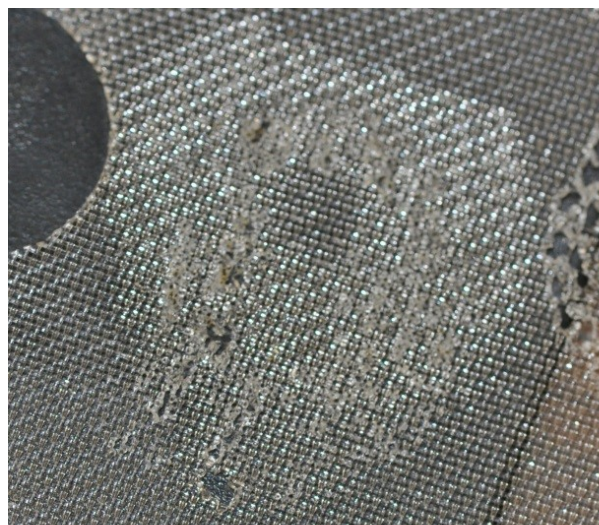
(b) High Power Nylon Mesh Deposition
