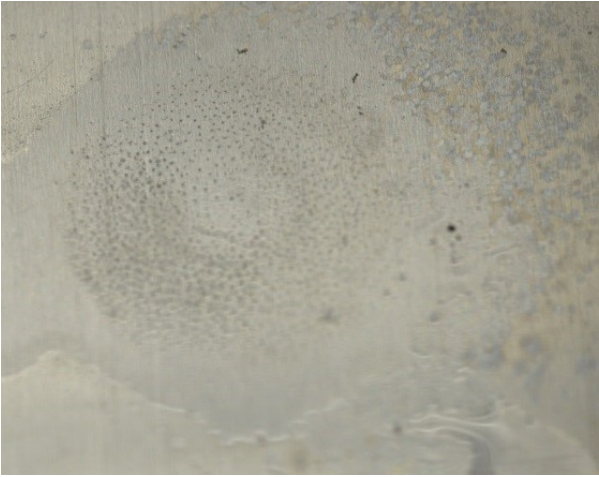
(a) Higher Powered Treatment on Stainless Steel Substrate with Black Specs
