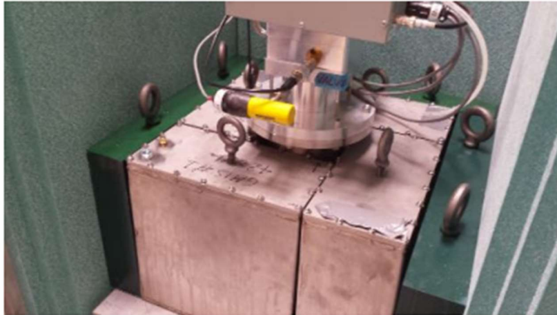
Figure 2.4 Photograph of the uranium target boxes and reflectors surrounding the neutron generator within the shielding enclosure. The east wall is removed. Approximate total uranium mass is 395 kg for the target sheets and 904 kg for the reflectors.
