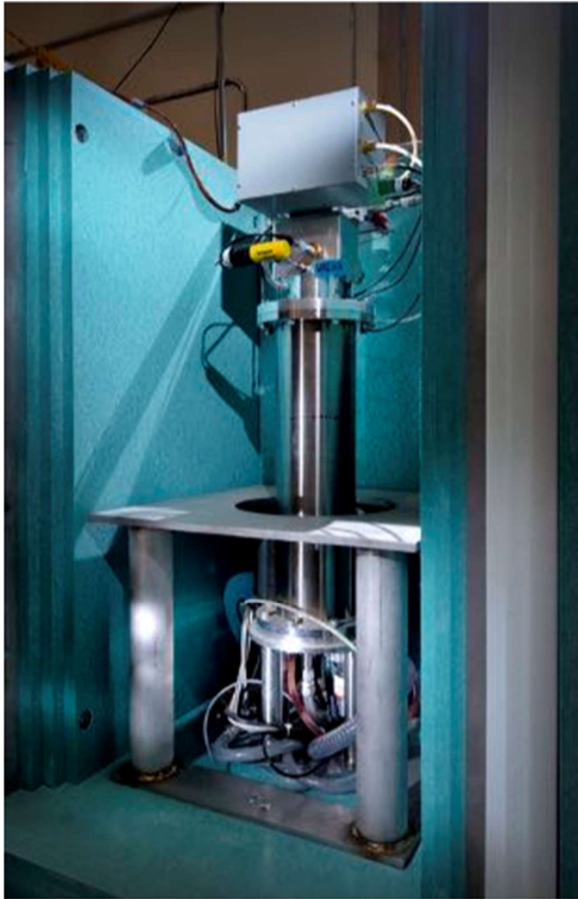
Figure 2.3 Photograph of the GMIS neutron generator and support features in shielding enclosure. The dashed line marks the apex of the generator's target and the mid-line of the absent uranium system elements. The east and top shielding layers are removed. The inner cavity dimensions are 60.96 cm X 60.96 cm X 121.92 cm. The exterior shielding dimensions (including removed lid) are 96.52 cm X 96.52 cm X 147.32 cm.
