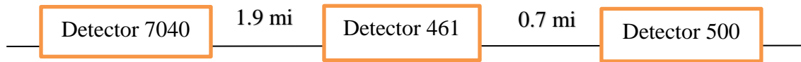
Figure 18 Example of a detector set up to calculate the segment length for detector no. 461
