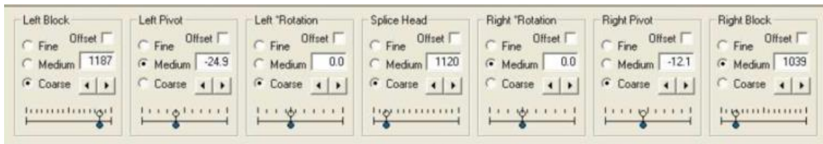
Figure 8. Vytran FFS2000 graphic user interface. Left block and right block control the left fiber and right fiber position, left pivot and right pivot are used to align two fibers, left rotation and right rotation are used to rotate two fibers, and splice head is used to move splice head position.
