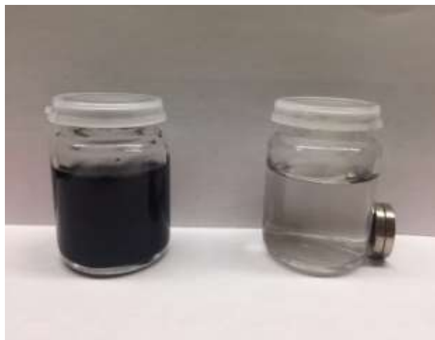
Figure S4.6. Magnetic separation of FA-BC in the aqueous solution under an external magnetic field.
