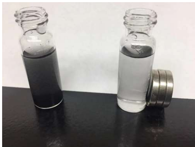
Figure S3.5. Magnetic separation of IA-BC 2.0 after SMX adsorption under an external magnetic field.
