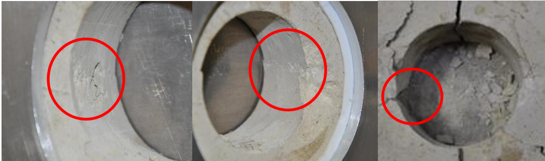
Figure 62. Borehole failure in center layers of the dismounted specimen in the large scale tests. Left: failure on the center of the left borehole wall. Center: failure on the center of the right borehole wall. Right: failure on the center of the left borehole wall.
